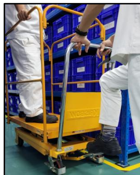
Fig. 3 Installation of safety frame on lift table
